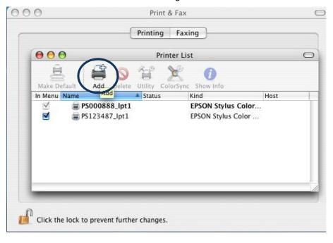
5. Enter the "Printer Type", "Printer Address" and "Queue Name" and select the "Printer Model" to setup the MFP Server. Click "Add" to continue.
